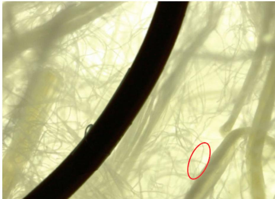
**Figure 21.** *Delignified Pineapple Fiber Compared to 28 Gauge Wire. The red circle is indicative of the exact fiber that was measured.*
