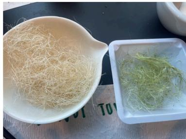
**Figure 4.** Decorticated fibers (sisal, left; pineapple, right)
