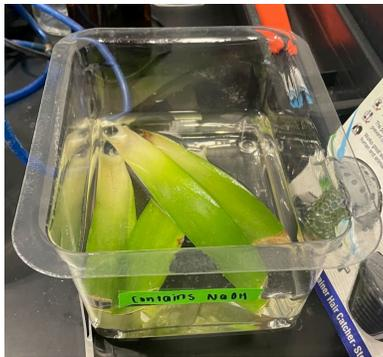
**Figure 2.** *Sodium Hydroxide bath to prepare for decortication*
