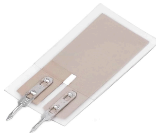
Figure 3. Piezoelectric Flexible Film Sensor. Image taken from Google Images.
