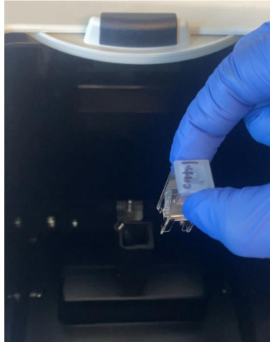
**Figure 6.** Transfer of sample cuvette into UV-Vis spectrophotometer
