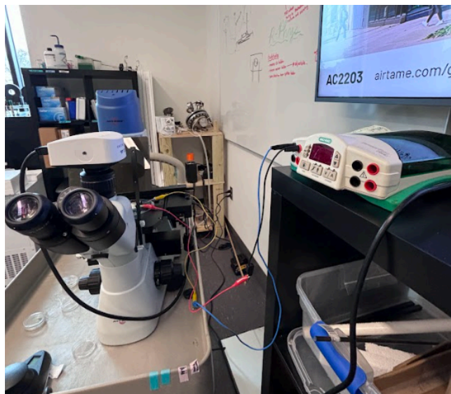
Figure 3. Electric Field Apparatus setup using Biorad power source and custom banana clips to ensure proper connection
