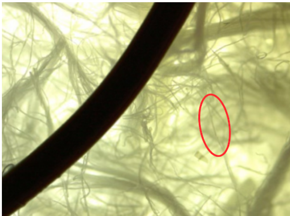
Figure 22. Delignified Sisal Fiber Compared to 28 Gauge Wire. The red circle is indicative of the exact fiber that was measured.
